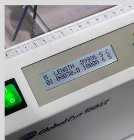
The Global Cut 100 is an electric cutting machine designed for cutting both round and flat material.
