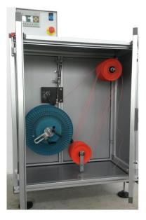
The SV4 machine is for unwinding spools, it is designed and manufactured entirely (mechanical, electrical and software) internally at SAVOTEC and it is complete of CE certification. Suitable for unwinding reels of cable tubes, sleeves, etc up to an outer diameter of 8 mm. Loading the coils is simple and fast with a system of rapid fixation of the coil on a 'support shaft. Thanks to an operator panel the speed, acceleration and deceleration of the rotation coil can be adjusted.
