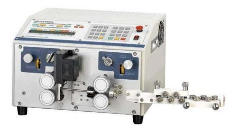
A cost effective and reliable machine with high speed and high productivity. Very easy to use protective membrane keypad and a large LCD display. All parameters such as cable lengths, stripping lengths, cable cross section, quantities and batch quantities are entered using the keyboard. Stepper motor driven wire transport with four driven wheels as well as stepper motor driven stripping knife, no blade change necessary.
